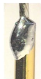
Unacceptable Excessive solder
