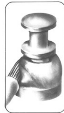
Unacceptable Excessive solder
