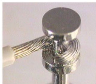
Unacceptable Insufficient solder joint
