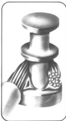
Unacceptable Insufficient solder
