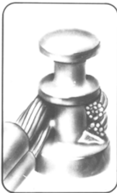
Unacceptable Insufficient solder
