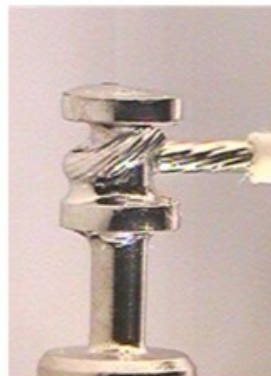
Unacceptable Insufficient solder joint
