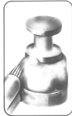
Unacceptable Excessive solder
